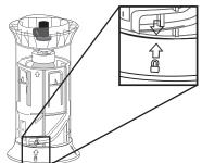
Step 4. Remove the flexible cap from the fluid connection. Attach the quick-fit connector to tubing if not already attached. Push the quick-fit connector downwards onto the shroud fitting until it clicks into place.
